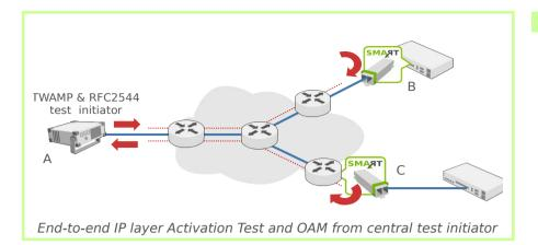
Upgrade IP networks with TWAMP and IP layer Service Activation Test capabilities using the Smart SFP  $^{\rm TM}$  module.
